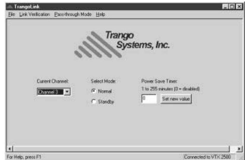
This TrangoLink interface screen shows that the transmitter is set to Channel 3, in normal mode (not standby), with the power-save timer set to zero minutes (secure standby). In this configuration, the transmitter will not reenter standby mode after awakening.
