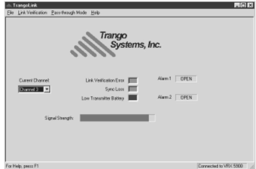
This TrangoLink interface screen shows the receiver set to Channel 3, both alarms open, and a low-battery condition on the transmitter.
