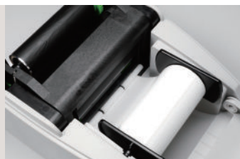
> Media Shaft Design for stabilizing paper
